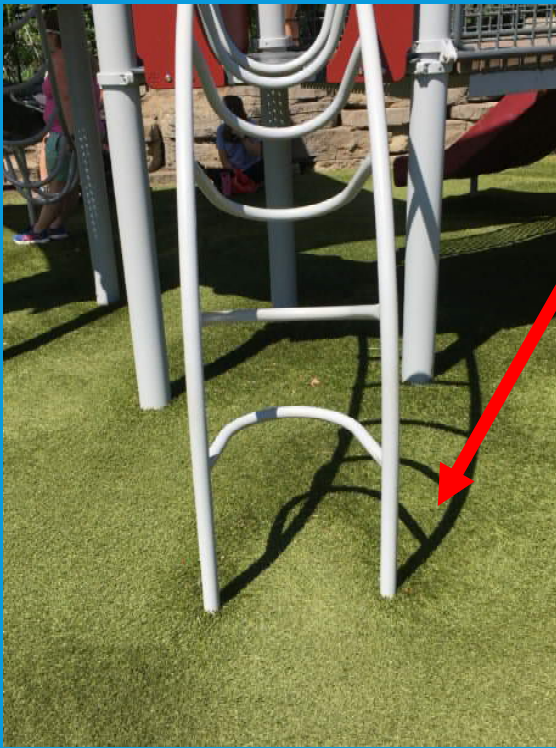
Matted down synthetic turf=can be a sign of Gmax/HIC failure! Potentially dangerous for falls
